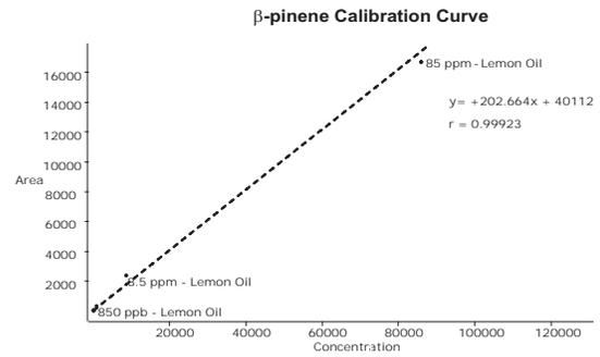
Figure 6: The calibration curve for  $\beta$ -pinene with concentrations from 8.5 ppb to 85 ppm.
