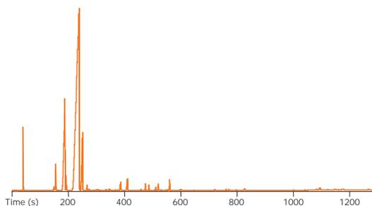
Figure 1: An optimized GC chromatogram for the TIC of 1  $\mu\text{L}$  of lemon oil at a split ratio of 300:1.
