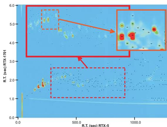
Figure 2: An optimized GCxGC contour plot of 1  $\mu\text{L}$  of lemon oil at a split ratio of 300:1. The inset is a magnification of an area which highlights the enhanced separation in the second dimension.
